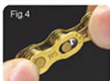
Fig.4 Press both halves of the MissingLink connector together.
