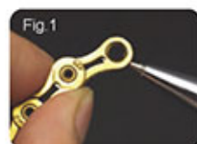
Fig.1 01. Fit chain with the correct length, clean bearing and lubricate.
