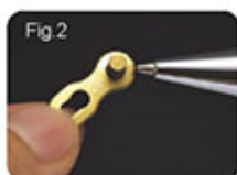
Fig.2 Do not forget to lubricate the pin.
