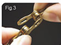
Fig.3 Insert both halves of the MissingLink into the chain ends.
