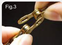
Insert both halves of the MissingLink into the chain ends.
