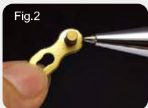
Do not forget to lubricate the pin.
