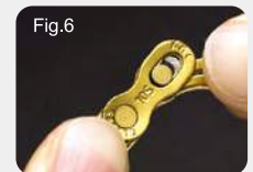
Opening: press both plates together while sliding the chain ends towards each other.
