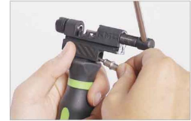
Accommodates all chain widths Additional storage space holds a second reversible pin.
