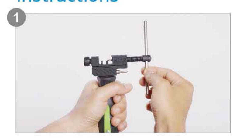
Rotate handle counterclockwise until de-riveting pin clears chain cradle, and rotate knob counterclockwise to allow space for chain.
