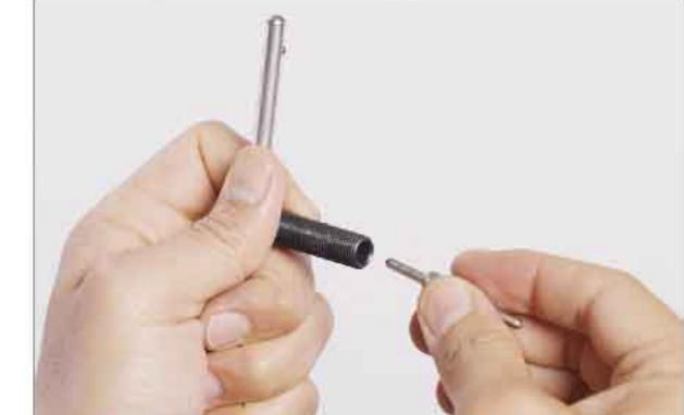
Pull the pin out of the handle. Rotate pin 180 degrees, and insert back into handle. Replace handle into chain tool body.
