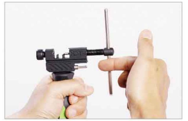
Rotate the handle counterclockwise.Remove entire handle with pin from chain tool body.
