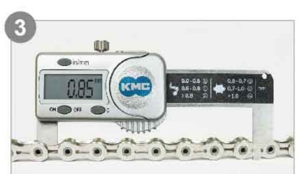
Turn on and press together as shown. Press "Zero" to calibrate.
