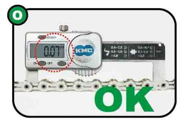
Hook on roller and insert into appropriate link (you may need to apply pressure). Look at the digital readout and refer to the next chart.
