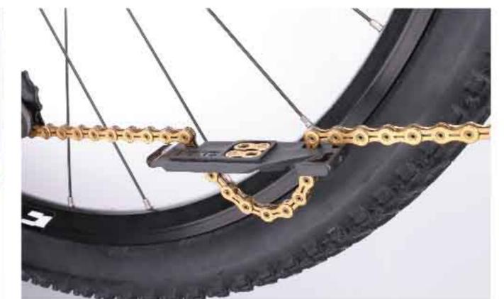
Chain hook: Hook one end of the Chain Aid onto chain. Next, press rear derailleur to loosen chain, allowing chain slack with the disassembly point in the middle, and then hook other end of Chain Aid onto chain.
