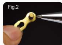
Do not forget to lubricate the pin.
