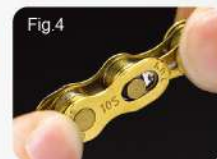
Press both halves of the MissingLink connector together.
