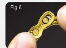
Opening: press both plates together while sliding the chain ends towards each other.
