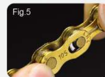
Lock in place by pulling the chain apart.
