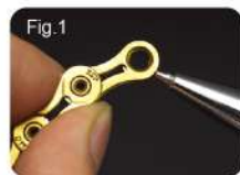
01. Fit chain with the correct length, clean bearing and lubricate.
